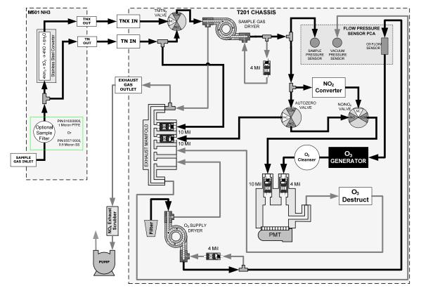
Figure 1-2. T201 and M501 NH<sub>3</sub> Pneumatic Flow
